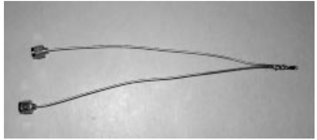
Figure 4: Low inductance wire fixture used to measure MLC capacitors.
